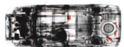
3. Dual Energy Auto Detect Image highlights suspicious objects in red
